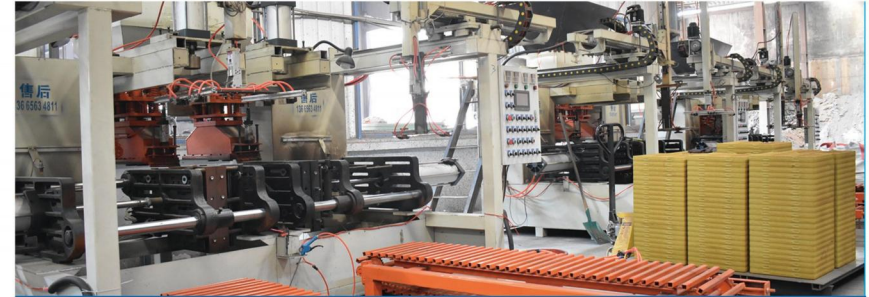
全自动750射芯铸造线（覆膜砂小球工艺） Fully automatic 750 core casting line (coated sand pellet process)
