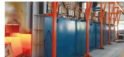
推杆式燃气淬火回火生产线 Pushrod gas quenching and tempering line
